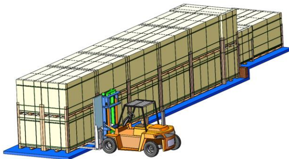
Vertical landscape package unloading with forklift
