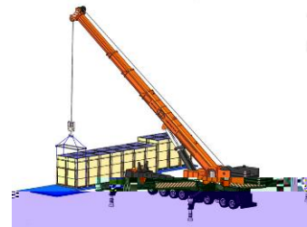
Vertical portrait package unloading with crane
